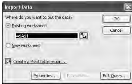
Figure 30-35. If you've already set up a query, you can turn it into a PivotTable by clicking Create A PivotTable Report.
