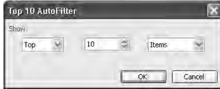
Figure 28-21. Use the Top 10 dialog box to zero in on the top or bottom n list elements.
