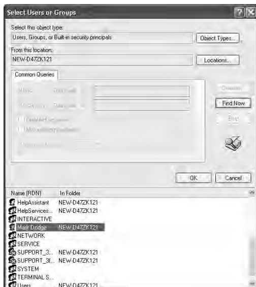
Figure 5-27. Click Add in the Permissions dialog box to add to your list of authorized users.
