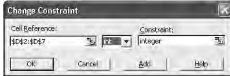
Figure 18-28. To specify an integer constraint, select the item labeled int in the drop-down list.
