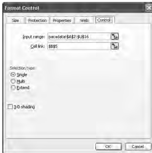
Figure 28-41. With the properties shown here, the list control box will display the items listed in pacadata!A2:U16. The number of the item selected (its position within the list) will be returned in cell B5.
