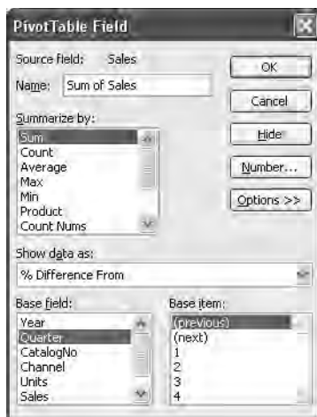
Figure 30-28. These settings will create a field that calculates percentage of change from the previous quarter.
