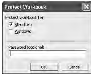
Figure 6-9. Choosing Tools, Protection, Protect Workbook helps insulate your workbooks from inadvertent modification.
